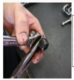
To get the plastic end off of the stock shifter, place a wrench against the big ball on the stock shifter, then use a pair of needle nose to pry the piece off of the stock shifter
