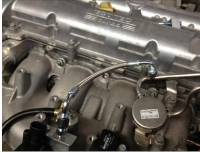
8. Install the supplied braided fuel line on the fuel feed fitting and then the new ZZP fuel rail; zip-tie all connections.
