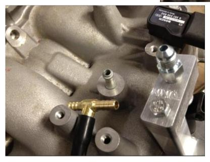
6. Using the supplied vacuum T, connect the intake vacuum port closest to the evap solenoid. This is the same port used for the BOV on the ZZP turbo upgrade kit.
