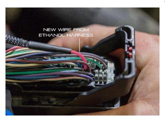
Install the pink wire from the ethanol sensor harness into pin 38 (or 70 for '16+). Pay attention to the orientation of the other pins so that the new wire/pin will lock into place properly. Reinstall the blue position cover, wire cover and plug the connector back into the ecm.
