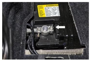
Battery access panel is located in the driver side trunk compartment
