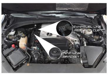
Remove the evap line bracket and evap line/fuel feed line bracket. You will not be reusing the evap/fuel feed line bracket.
