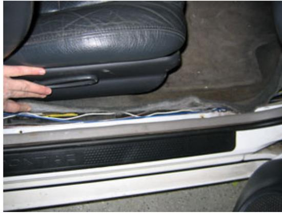
Remove the trim and pull the carpet back an inch or two. Run the blue wire that is coming through the firewall under the carpet towards the back seat. Remove the lower part of the rear seat by pulling the two clips under the front. Slide the wire underneath the rubber insulation toward the fuel pump trap door. The fuel pump door is located behind the flip down part of the upper rear seat.
