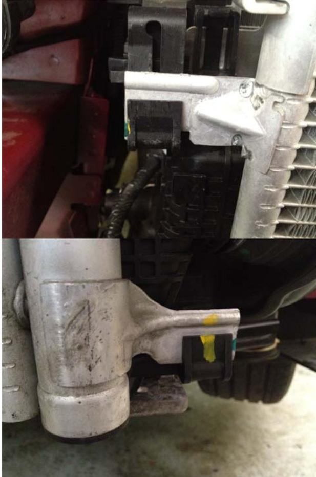
13. (Automatic only) Now, remove the transmission cooler from its brackets and swing it away from the radiator. The transmission cooler is removed the same way you removed the a/c condenser.
