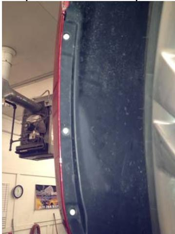
2. Next, remove the outer push clips on each side of the vehicle that attach the bottom spoiler to the bumper cover.
