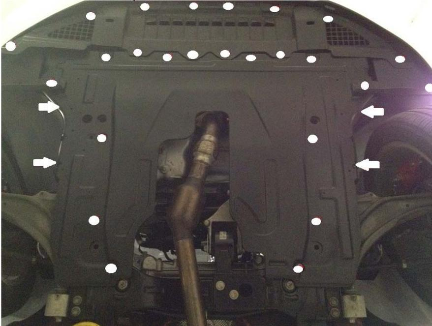
4. Once you have removed the plastic shields you gain access to the lower hot side charge pipe. Using a flat blade screw driver or an 8mm socket remove the lower hot side charge pipe.
