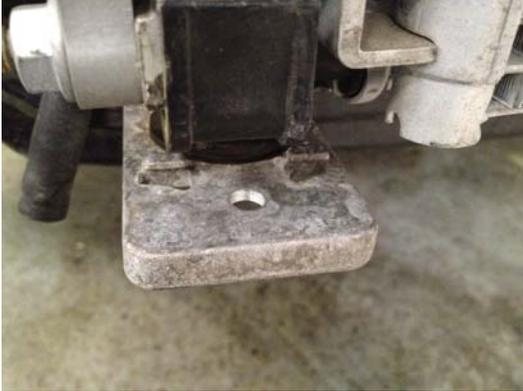
2. Install the new ZZPerformance Intercooler using the supplied 8mmx1.25 bolts and nuts. This will require a 13mm wrench and socket. You will have to bend the a/c line out of the way to make room for the new intercooler. Don't worry you will not break the lines if you use some common sense. The metal is soft and requires no sharp tools just light pressure.
