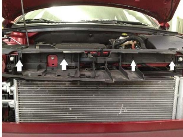
9. Remove the plastic covering the radiator, intercooler, and condenser. **You will not be re-using this.**
