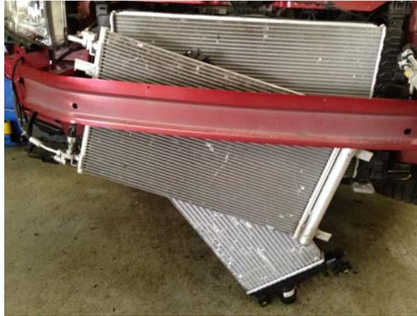
15. Once you have removed the IC you can install the a/c condenser into the same location that the Intercooler was removed from.
