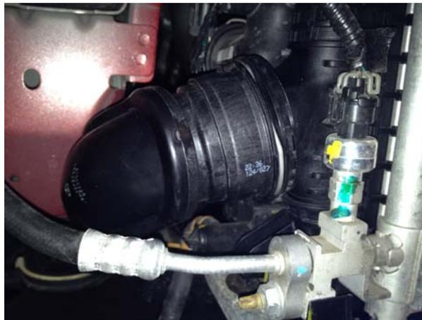
11. Next, remove the upper charge pipe. **You will not be re-using this pipe.**
