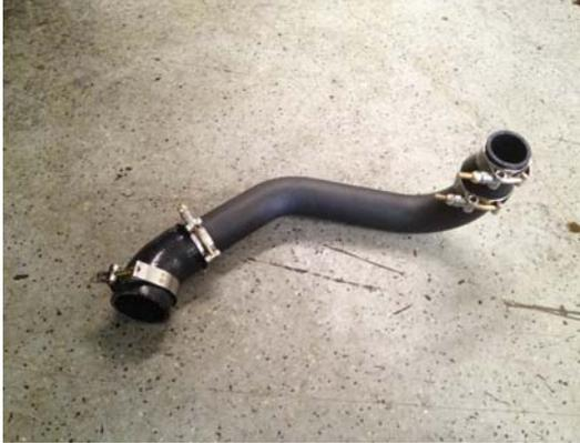
5. Next, move onto the installing the upper charge pipe. Remove your map sensor from your factory charge pipe and install it in your new ZZP pipe. Removing the sensor requires a T20 torx bit and installation requires a 5mm allen wrench. The extra port on the map sensor pad is for reading boost or what ever you decide to do with it. **If you are not going to use the port make sure the pipe plug is installed to prevent a boost leak!**
