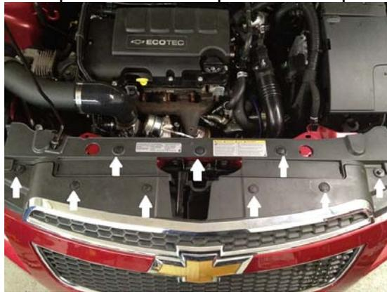
4. Now, carefully pull the bumper cover off of the bracket holding it to the fender starting on the side closet to the wheel. Repeat on opposite side.
