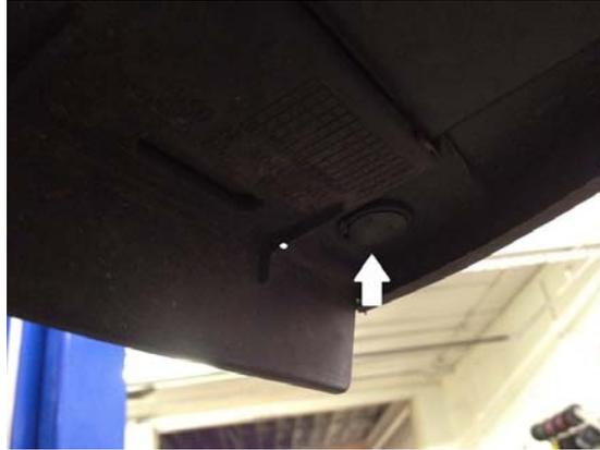
3. Moving to the top of the vehicle remove the two bolts from the bumper cover using a 10mm socket. Next, remove the four push clips across the top of the bumper cover.
